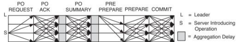
Fig. 2. Fault-free operation of Prime ( f = 1 ).
