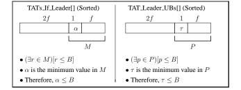
Figure 5: The value of TAT\_acceptable  $(\tau)$  computed at any correct server converges to a value where  $\tau \leq B$ . The sets M (left side) and P (right side) contain the f+1 highest values in their respective vectors. M must eventually contain at least one value, v, reported by a correct server, where  $v \leq B$ . Thus,  $\alpha \leq B$ . Using a parallel argument, the right side shows that  $\tau \leq B$ .
