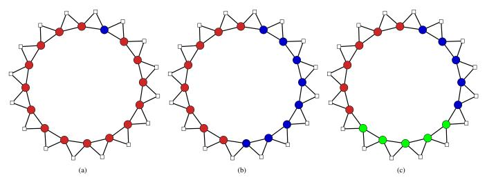
Fig. 6. Ring topology of 16 clients and 16 routers which highlights difference between optimizing (a) expected client connectivity, (b) probability of Paxos progress, and (c) probability of BFT progress.
