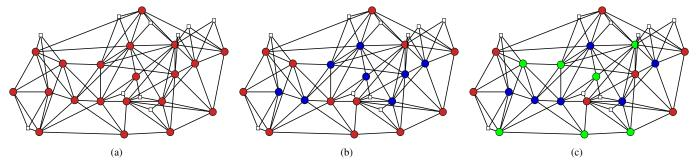
Fig. 2. Optimal assignments on case study topology: (a) one variant assignment achieves 0.9 expected client connectivity, (b) two variants assignment achieves 0.985 expected client connectivity, (c) three variants assignment achieves 0.997 expected client connectivity.
