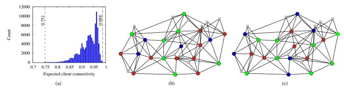
Fig. 3. Random and greedy assignments on case study topology: (a) histogram of expected client connectivity of 100,000 random assignments with vertical lines displaying the lower and upper bounds, (b) random assignment achieving 0.881 expected client connectivity, and (c) greedy assignment achieving 0.992 expected client connectivity.
